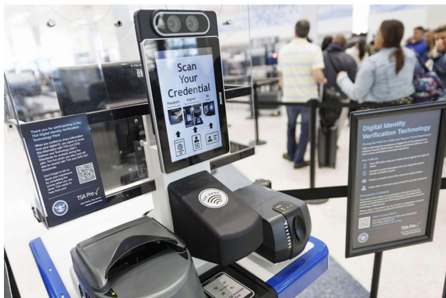
FIGURE 4: TSA CREDENTIAL AUTHENTICATION TECHNOLOGY TYPE 2 (CAT-2) SYSTEM TO WHICH TRAVELLERS CAN PRESENT THEIR DIGITAL LICENSE VIA NEAR-FIELD COMMUNICATIONS (NFC) FOR IDENTIFICATION PURPOSES TO GAIN ACCESS TO THE SECURITY CHECKPOINT IN THE AIRPORT.
